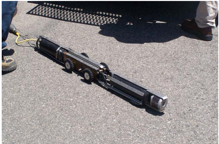
Photo 5: The self-propelled sewer inspection camera
