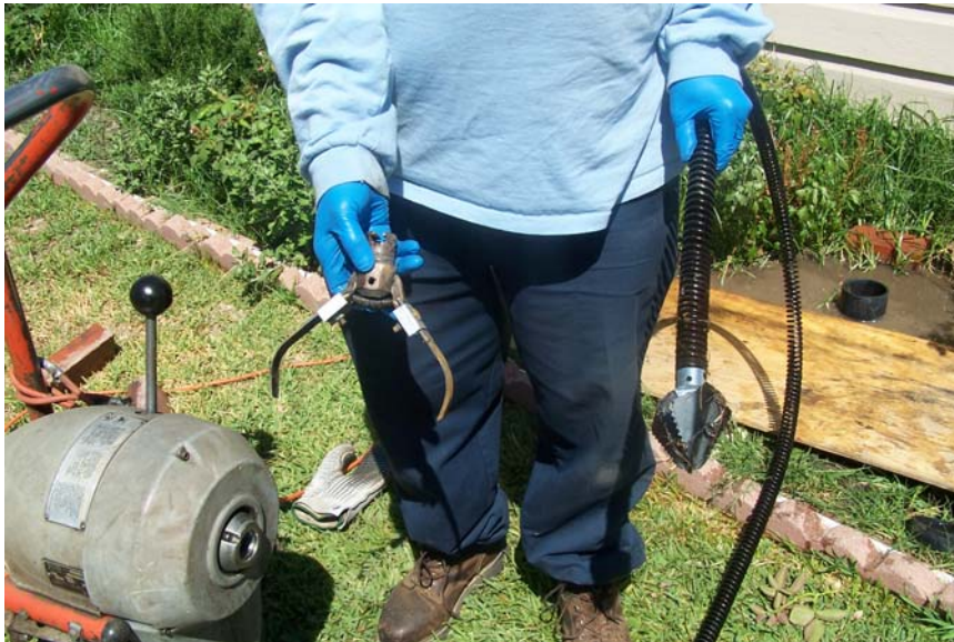
Photo 10: The rodding machine operator shows the two types of cutting heads: the finisher on the left and the bullet on the right.
