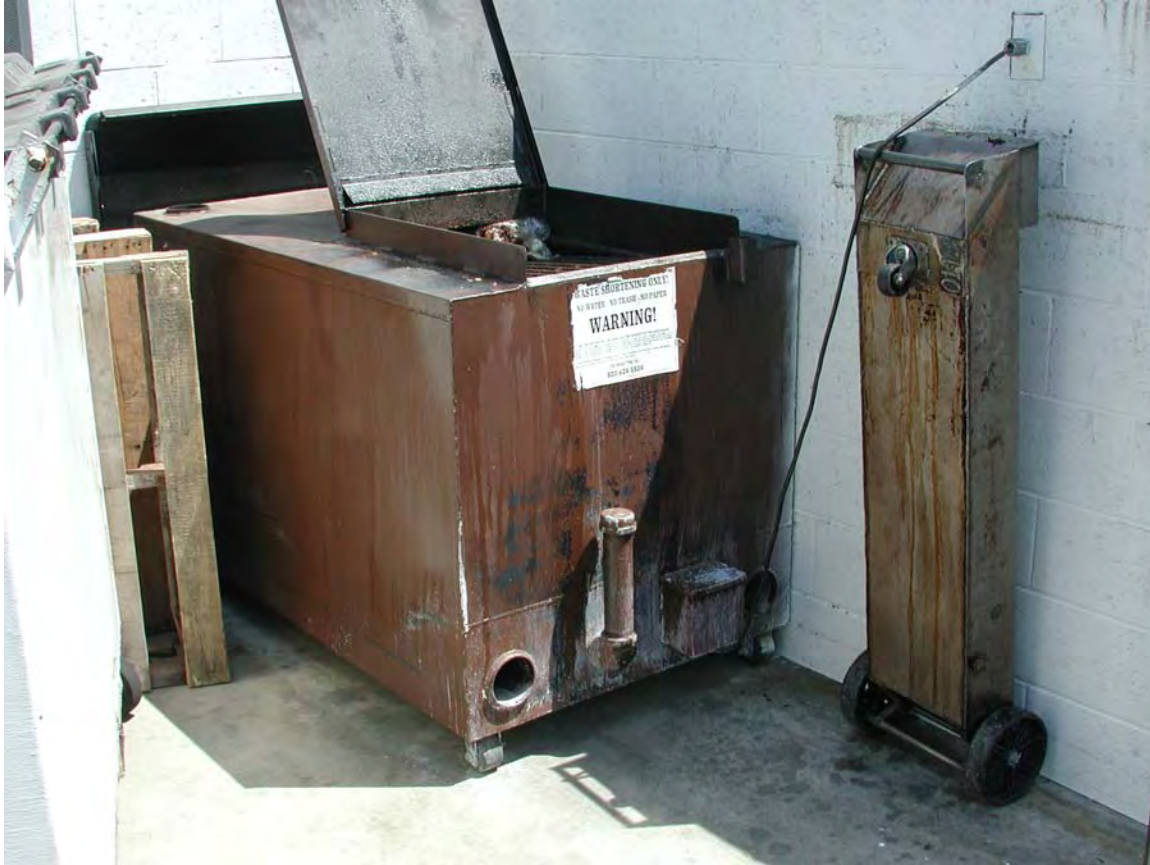
FIGURE 6-4 Yellow Grease Recycling Bin (Courtesy of County Sanitation Districts of Los Angeles County)
