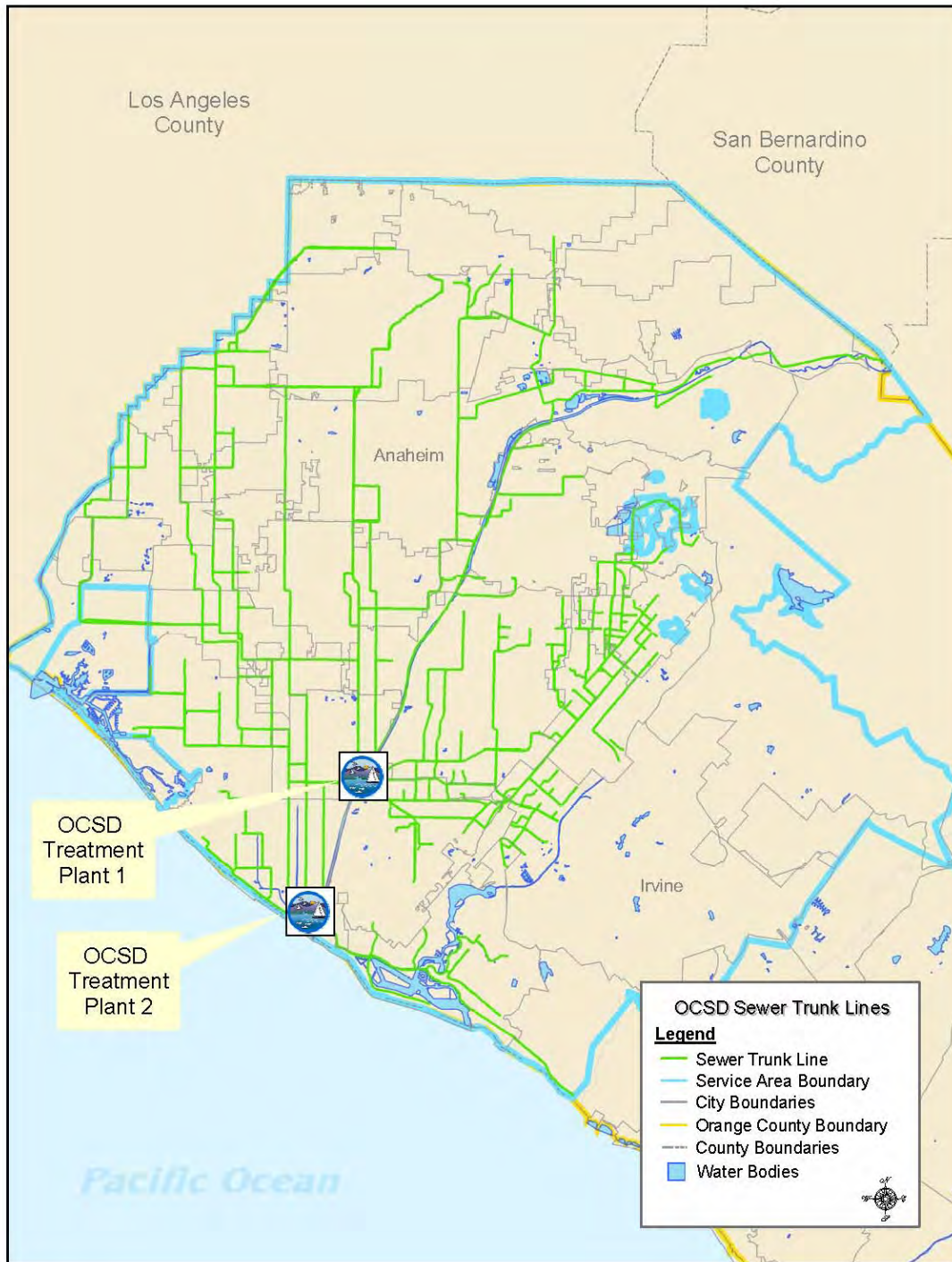
FIGURE 5-1 OCSD Service Area and Sewer Lines
