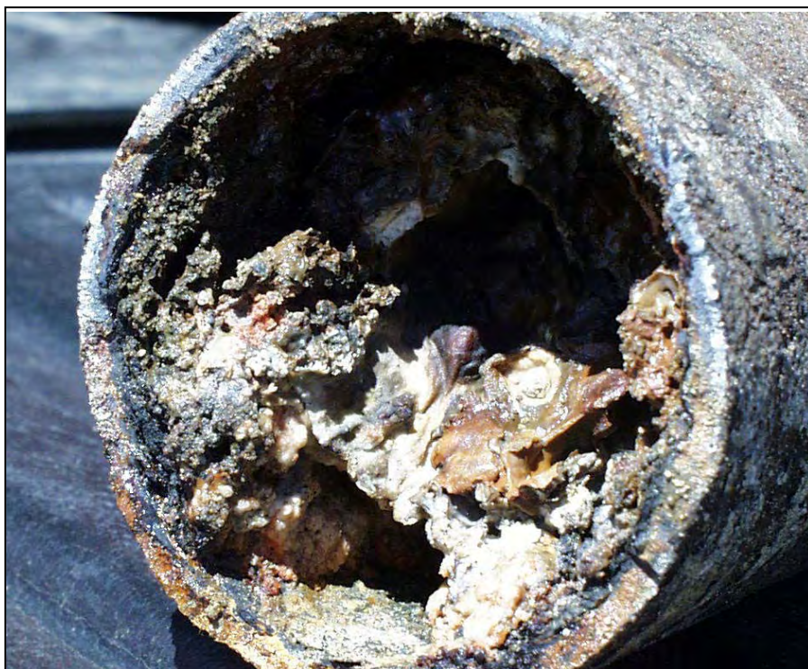
FIGURE 2-1 Sewer line grease blockage (Courtesy of Monterey Regional Water Pollution Control Agency)
