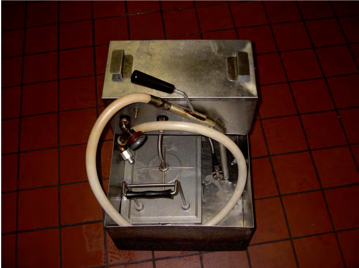
FIGURE 6-6 Portable Fryer Grease Transfer Container
