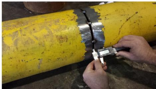
Figure 6. Measurement of the Annular Gaps
